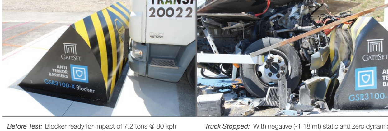
Continuity of Services: Blocker remained intact and fully operable after impact
