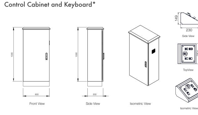
\* Above cabinet measurements are for an outdoor cabinet for standard three group configuration. Subject to change depending on design or project needs without prior notice
